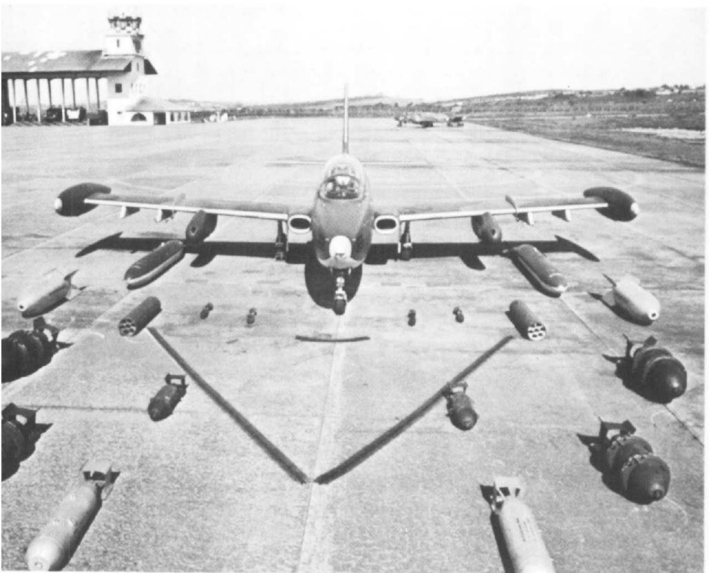
The EMB-326GB Xavante (air force designation, AT-26). Ground attack aircraft built by Embraer under license from Aeronautica Macchi of Italy; powered by a Rolls Royce turbojet engine. Photographs Courtesy Office of the Air Attaché, Embassy of Brazil, Washington.
